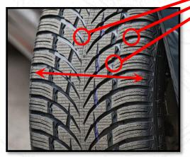
Info: If you pay attention to small elevations in the tread grooves, the so-called <u>Tread Wear Indicator</u>, you can determine the height of 1.6mm.
